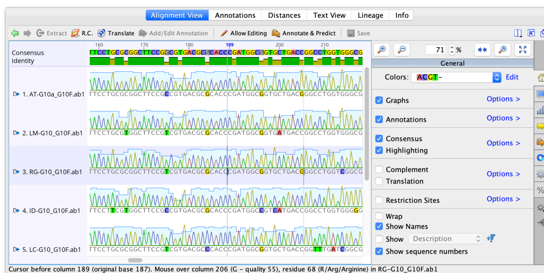
Figure 5.6: A sequence alignment containing chromatograms, with quality scores enabled
